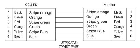
1,2 wires - TALK/ 3 wire - DATA/ 4 wire - POWER (VCC)/ 5 wire - VIDEO/ 6 wire - GND
