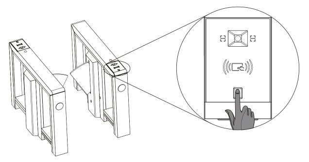
**Recommended fingers:** It is recommended to use index, middle, or ring finger for registration and avoid using the thumb or little finger, as they are difficult to accurately press onto the fingerprint reader.
