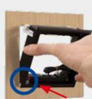
3. Insert the FlatMount Frame into the opening. Make sure that the red knob is on the lower left corner and that the arrow on the red knob points at the "open lock" icon. Insert the lower left edge of the frame first, then follow with the lower right edge. After that, slightly pull the lower part of the frame back out. This causes the upper part of the frame to "fall" into the opening.
