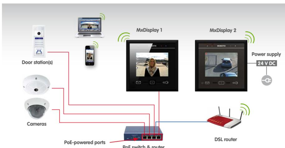
MxDisplay 1 is connected to a safe PoE connection and serves as remote station for the door station as well as WiFi access point for additional remote stations (iPhone, iPad). MxDisplay 2 is farther away and uses the WiFi network of the DSL router. It is used primarily as video management system to monitor and configure the installed cameras.
