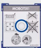
Set the protective cardboard cover (included with the delivered parts) into the housing before pushing it into the wall cavity. This prevents cement from entering the interior of the housing. After you have installed the housing into the wall, you can easily remove the carton by pushing through the pre-cut opening and pulling it out.
