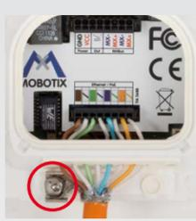
**Note:** To remove a wire, unlock the terminal by pressing with the screwdriver (included with delivery) into the opening above the wire. Then pull out the wire.
