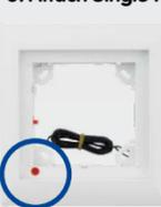
**On-wall/in-wall:** When attaching the frame, make sure that the arrow on the red knob (theft protection) points at the "open lock" icon and that the frame is positioned in such a way that the red knob is on the bottom left corner of the frame.
