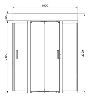
Concrete Base to specification at least fck (cube) 30N/mm2 of resistance. Base to be flat and level to  $\pm$ -5mm over footprint area. Dimensions to be >  $2050 \times 2050 \times 150$  deep min. (units in mm).
