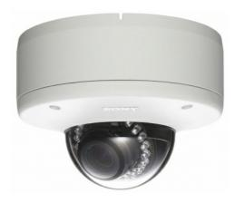
OVERVIEW The SNC-DH260 is an outdoor vandal-resistant high definition (1080p, supporting H.264 at 30fps) 3 Megapixel minidome camera with True Day/Night function, IR Illumination, DEPA and ONVIF compliance. It supports dual streaming and triple codec encoding.
