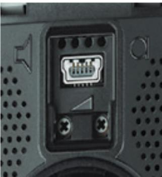
Mini-USB connection and loudspeaker/microphone volume adjustment
