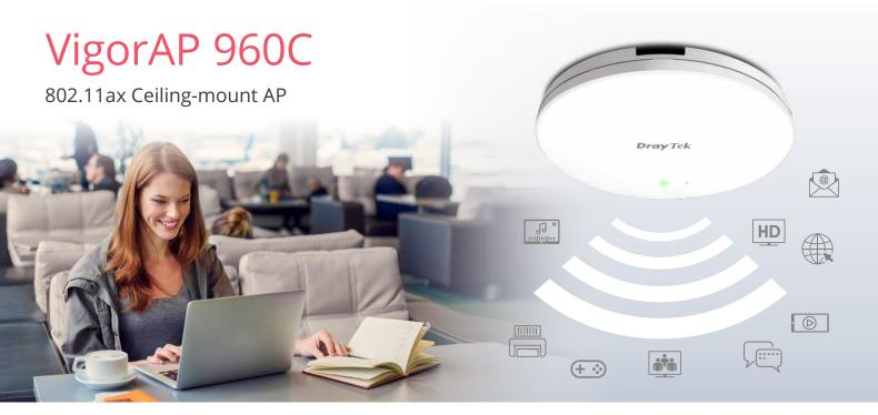
VigorAP 960C is an 11ax ceiling-mount wireless access point. With wire-liked speed up to 1.2 Gbps in 5GHz band and 600Mbps in 2.4GHz, it's suitable for high density environments. It can be cloud-managed by VigorACS, and also act as the mesh Root AP to manage up to 7 mesh node APs in LAN.
